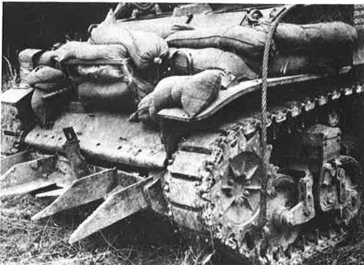
A tank equipped with teeth for making openings in Normandy hedgerows during World War II. The "Arsenal of Democracy" produced for itself and its allies 18 million rifles, pistols, and rapid fire weapons; 2½ million trucks and tracked vehicles; 87,000 tanks; 300,000 aircraft; 61,000 pieces of heavy artillery as well as millions of tons of bombs, shells, explosives, foodstuffs, clothing, and other materials.
